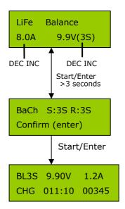
The value on the second line sets a charge current and the voltage of the battery pack. Press the START/ENTER button, and then press the **DEC or INC** to set value. After setting the current and voltage press **START/ENTER** button for more than 3 seconds to start the process. (Charge current: 0.1~8.0A, Voltage: 1~6 series)
