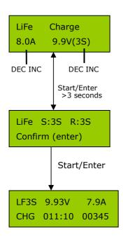
The value on the second line sets a charge current and the voltage of the battery pack. Press the START/ENTER button, and then press the **DEC or INC** to set value. After setting the current and voltage press START/ENTER button for more than 3 seconds to start the process. (Charge current: 0.1~8.0A, Voltage: 1~6 series)
